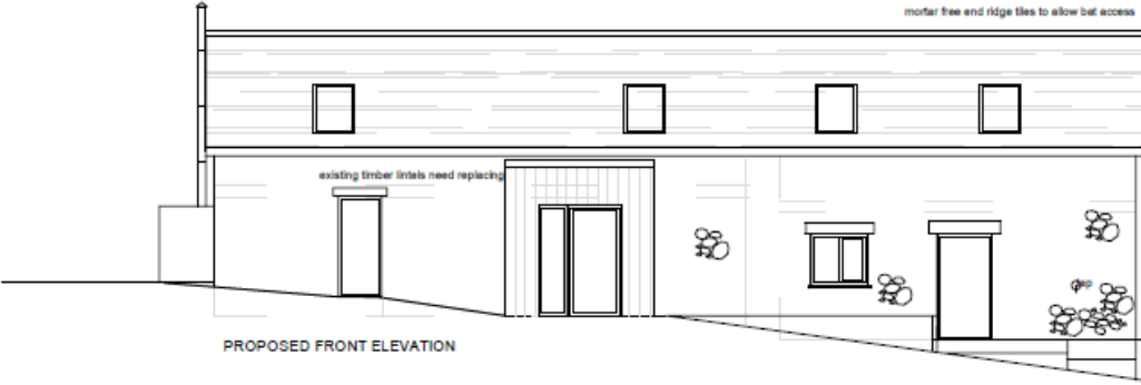
mortar free end ridge tiles to allow bat access
